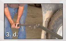
3. d. Push down, hand-overhand with light pressure, on end of torque wrench handle. Torque lug nut to manufacturer's specifications.
