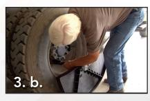
3. b. Install socket on the lug nut, slide Torque Fin® on the extension until it touches side wall of the tire.
